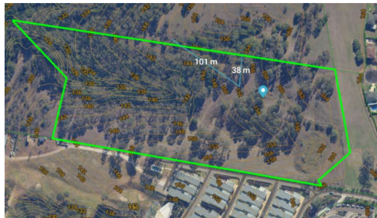
Figure 2.9 – Northwest slope validation from Building R4 out 101m
